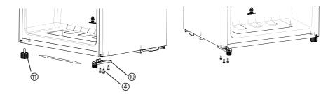
4. Dismantle the adjustable foot⊕, positioning bolts⊕and lower hinge⊕, then exchange the parts of right and left sides and later use the reverse method to install the adjustable foot and positioning bolts.
