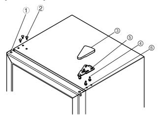
1. Change the installation location of the upper hinge sof the cooler, then the opening direction of the door could be changed at will. Please follow the following instructions for the change of the opening direction of the cooler's door (for instance: from right-handed door): close the glass door of the cooler, use a blade to remove the axle sleeve() and rivet() carefully, loose the mounting cover() of the door hinge and three positioning bolts() and remove the upper hinge() and axle sleeve().
