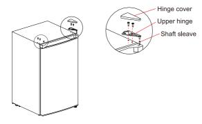
3)Remove the door first, then remove the lower hinge assembly and levelling foot, interchange the positions of the lower hinge assembly and levelling foot and install them.
