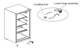
4)Install the door on the lower hinge assembly, and then install the upper hinge, hinge cover, shaft sleave, pins and hole cap in sequence.
