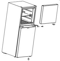
4) Remove the refrigerating door, remove the bottom hinge and adjustable foot of the other side.
