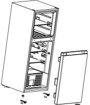
6)Place the refrigerating door from top to bottom, take out the gasket from the plastic bag in the instructions and put it into the axle hole on the left side of the refrigerating door, as shown in the picture. Fix the center hinge with screws and install the studs.
